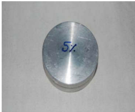
Pictorial view of sample containing 5% offlyashby weight for hardness test
