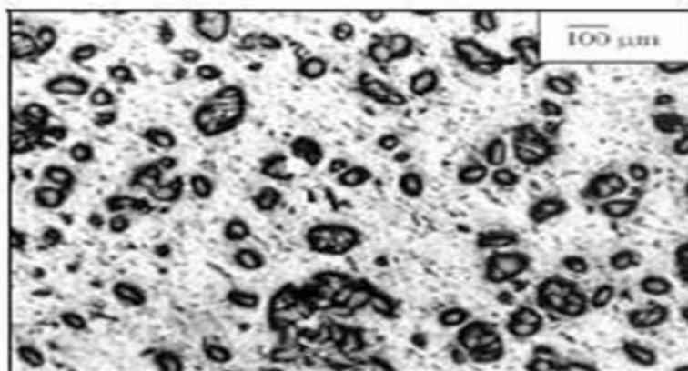
Fig.1. Photo Micro-graphic image of Al-SiC<sub>p</sub>
