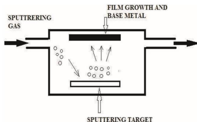
Fig.4. Conventional sputtering process [4]
