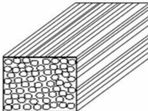
**Fig. 3.** Long fiber reinforced fiber.
