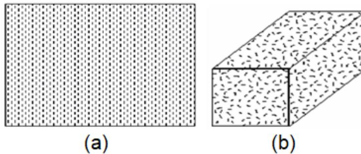
**Fig. 2.** Short fiber reinforces composite (a) Aligned and (b) Random.
