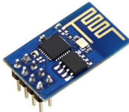
**Figure 7. ESP8266-01 Wi-Fi Module**
