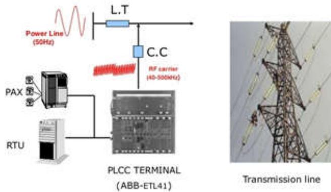
**Figure 1. Block diagram of PLC**
