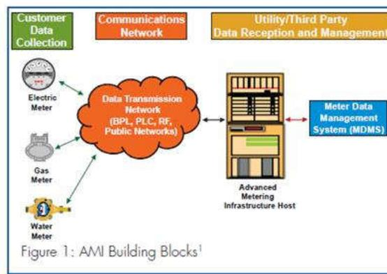
**Figure 3. Advanced Metering Infrastructure Block Diagram**
