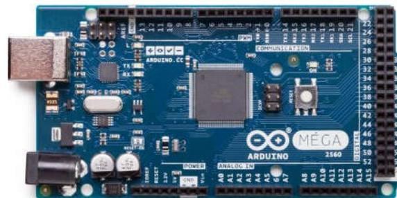
Figure 5. Arduino Mega with Atmega 2560
