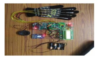
Fig 4: Sensor part of the system with processing unit, Audio playback module and GSM module
