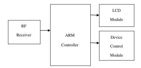
Fig 2: Block Diagram of Receiver Section
