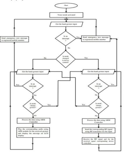
Fig 3: Working Diagram for Gesture Vocalizer for Deaf-Dumb
