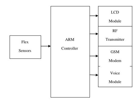
Fig 1: Block Diagram of Transmitter Section
