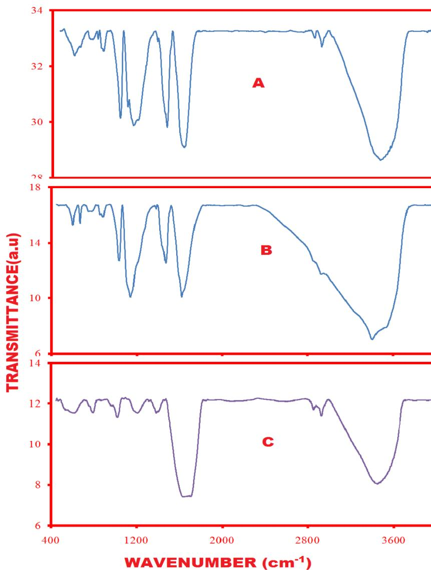
Fig. 3. 1 FT-IR Spectra of (A) PFR, (B) PFR blended with 20 % (w/w)
