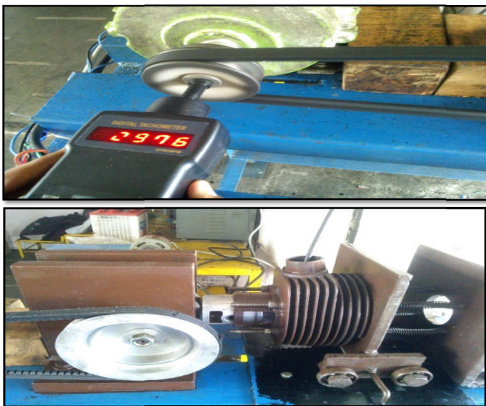
Fig.2: Measurement of Engine Speed with TACHOMETER at Motor Shaft
