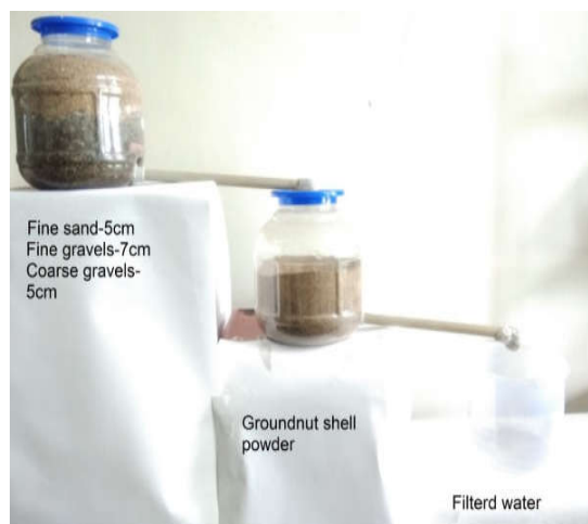
Fig 2. Set Up Of Filtration Of Groundnut Shell Powder
