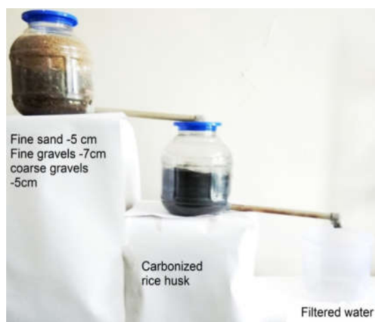
Fig 1. Set up of filtration for Activated Rice Husk
