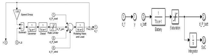
Fig.2.Conventional generator (Small Power System) model
