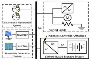
Fig. 1. Structure of microgrid with attached storage system.
