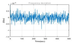
Fig. 12. Frequency deviation with control and maximum battery power
