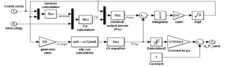
Fig. 4. Wind turbine generator model
