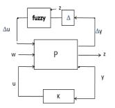
Fig 5. Control configuration for  $\mu$  –synthesis with Fuzzy pc
