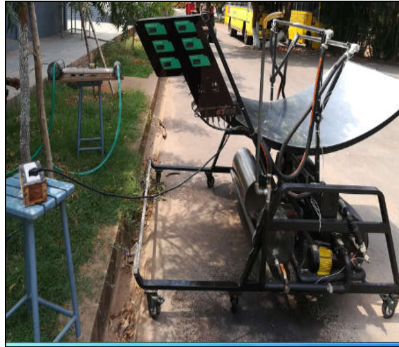
Fig. 2.5. Experimental setup with Solar Parabolic Collector
