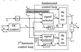
Fig.3. The adapted series converter control
