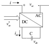
Fig.4. The simplified diagram of a series converter The voltage  $v_{se^*}$  is the control voltage for the series converter generated by the control, and the voltage injected by the series converter is given by:  $v_{se} = v_{se}*v_{de}$ . As the switching frequency of the converter is much larger than the grid frequency, the current at the dc side can be approximated to [4]:
