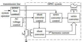
Fig.2. Block diagram of the control of a DPFC
