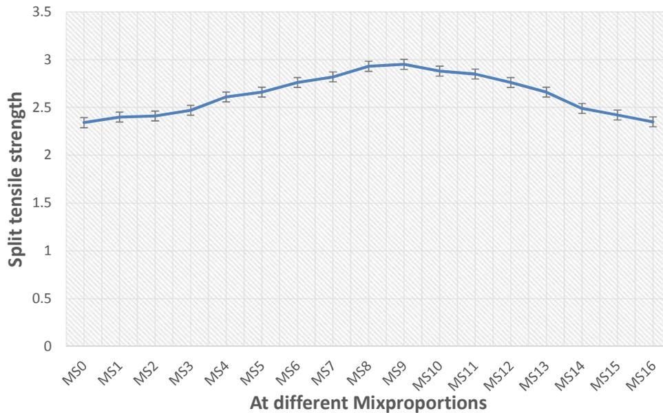
**Fig. 4 Split tensile strength after 28 days**
