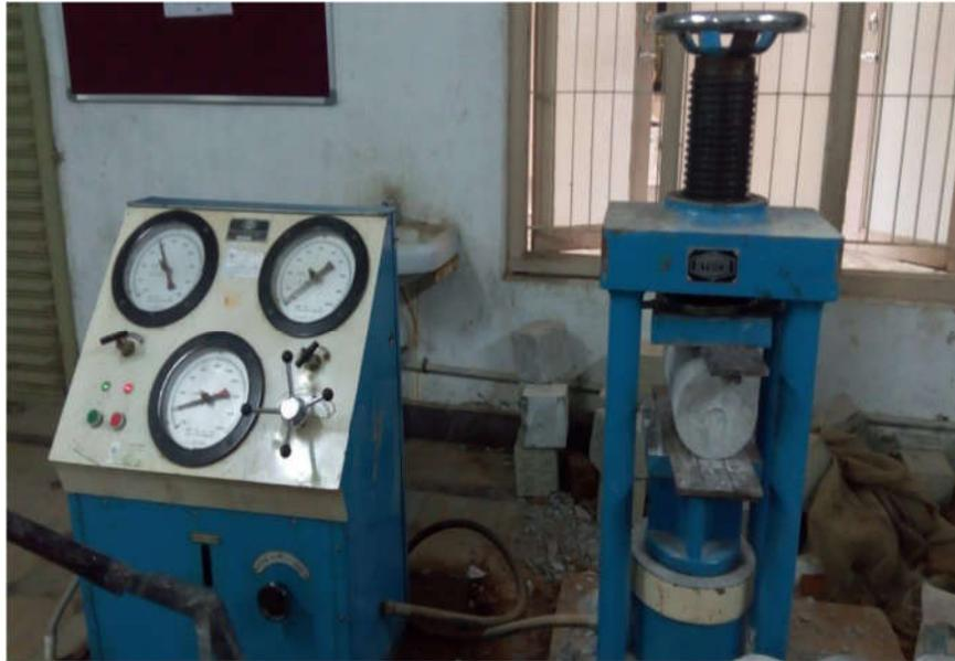
Fig. 2 Experimental set up to find split tensile strength of concrete
