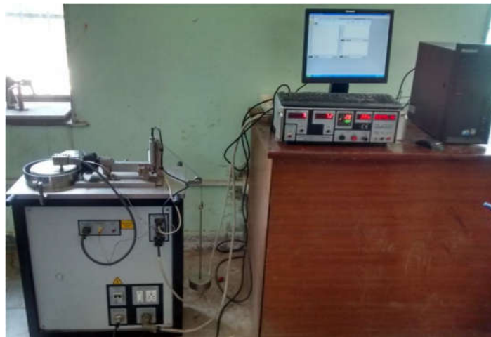
Figure 3. Complete Arrangement of pin on disc.
