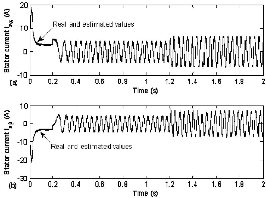
Fig 8. The actual and estimated stator currents
