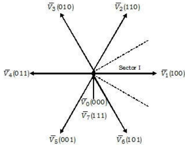
**Fig. 2 Inverter voltage space vectors**
