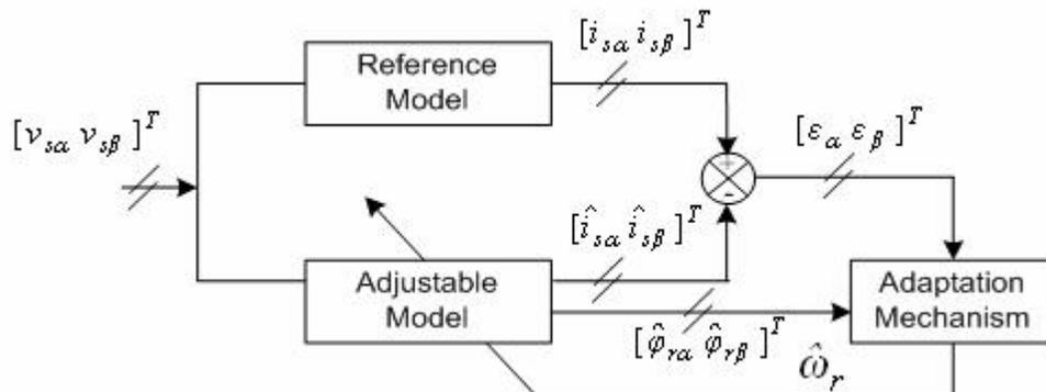
**Fig 3. Schema of the rotor speed estimation based on MRAS structure**
