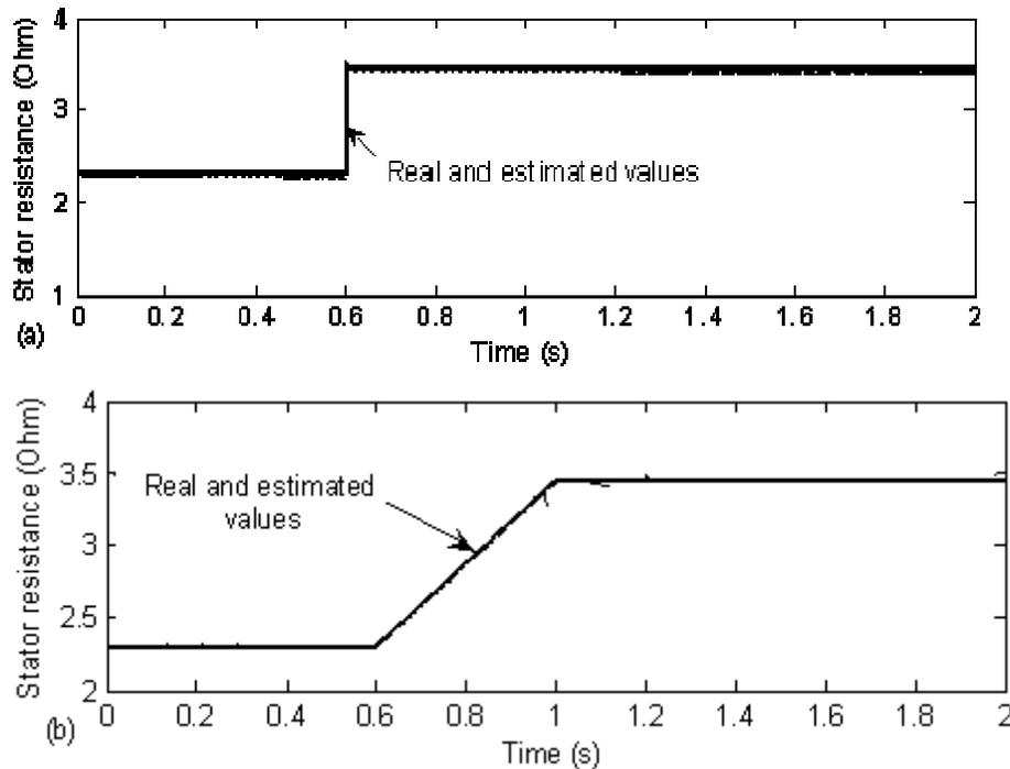
Fig 11. The actual and estimated stator resistance, (a) Abrupt variation, (b) Smooth variation
