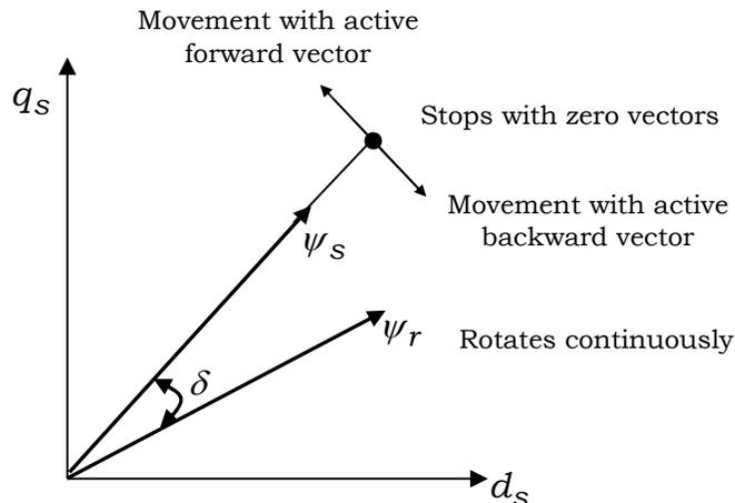
**Fig. 1  $\bar{\psi}_s$  movement relative to  $\bar{\psi}_r$  under influence of voltage vectors**
