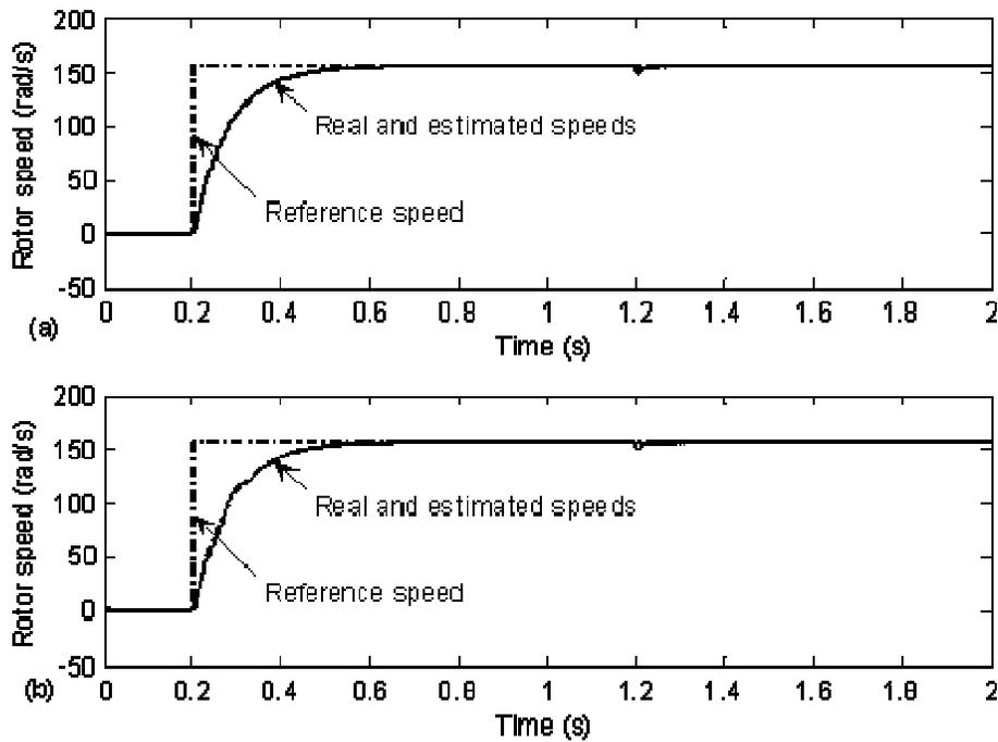
Fig 10. The actual and estimated speed (a) using the EKF, (b) using the MRAS
