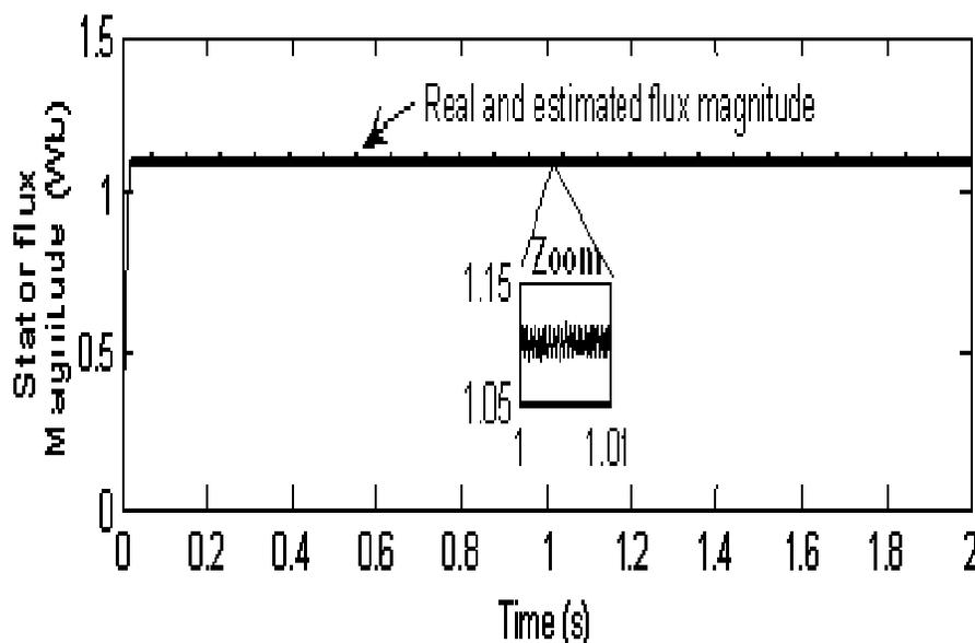
Fig 7. The stator flux magnitude
