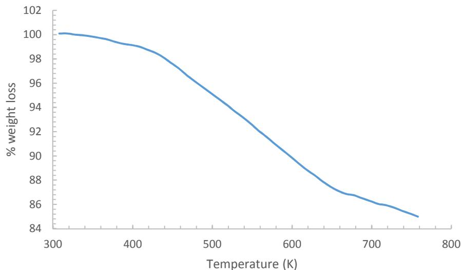
**Figure 2.** TGA of MW-CNT at the heating rate of  $10 \text{ K} \cdot \text{min}^{-1}$
