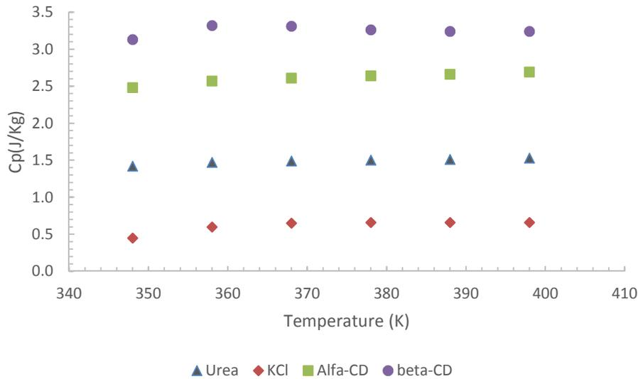
**Figure 1.** Specific heat capacity data for the standards urea, KCl,  $\alpha$ -CD, and  $\beta$ -CD as a function of temperature.
