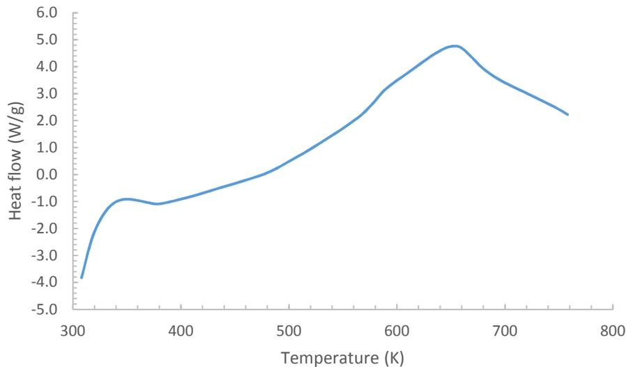
**Figure 3.** DSC of MW-CNT at the heating rate of  $10 \text{ K} \cdot \text{min}^{-1}$
