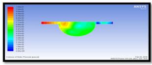
According to the pressure plot the maximum pressure value 1.09e-01 Pa and minimum pressure value 5.47e-03. The maximum pressure at inlet condition of combustion chamber and minimum pressure value at outlet conditions of the combustion chamber.
