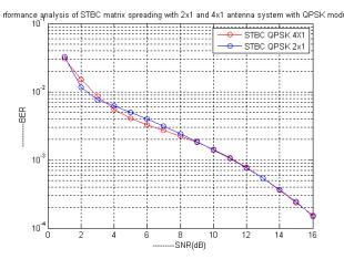
Figure 2.1 BER for STBC permutation for QPSK signaling for 4 transmit antennas, and 2 transmit antennas
