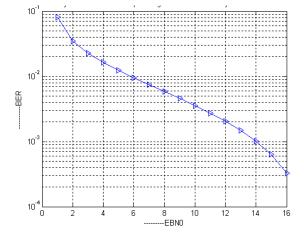
Fig.2 Performance analysis of MIMO-CDMA system employing permutation spreading based on STBC code while considering random channel path gains for 2x1 antenna system with BPSK modulation
