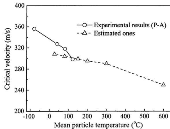
Fig. 4 Shows the variation of critical velocity with mean particle temperature [18].
