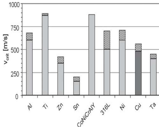
Fig. 2 Experimentally determined critical velocities of various spray materials. The error bar accounts for differences caused by the range of available powder purities [8].
