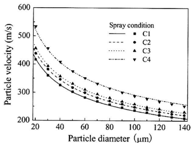
Fig. 3 Shows the variation of particle velocity with particle size under different spray condition [18].
