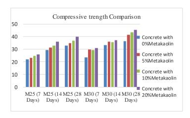
Fig. 8.1: Comparison of Compressive strength of Conventional Concrete and Concrete with Metakaolin
