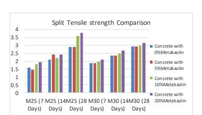
Fig. 8.2: Comparison of Split Tensile strength of Conventional Concrete and Concrete with Metakaolin
