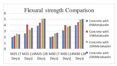
Fig. 8.42: Comparison of Flexural strength of Conventional Concrete and Concrete with Metakaolin
