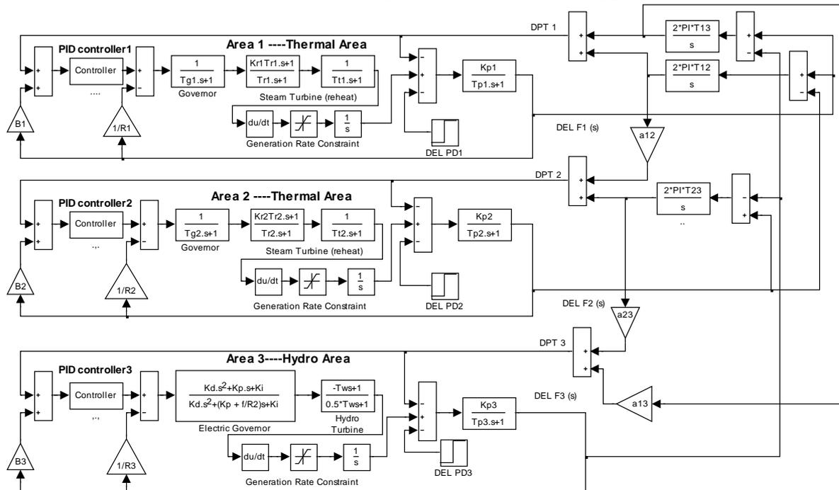
Fig. 1. Transfer function model of model of three-area hydro-thermal system with generation rate constraint
