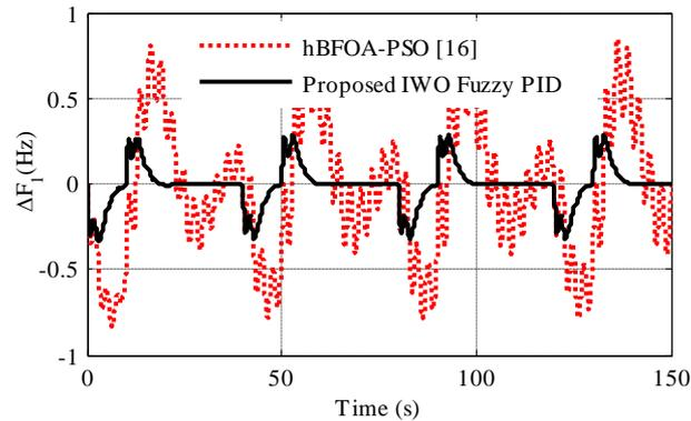
Fig.5 Frequency deviation of area-1 with pulse load pattern
