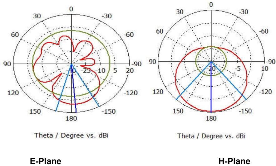
**Figure 10. Simulated Radiation Patterns in Different Cut Planes at 30.916 GHz.**
