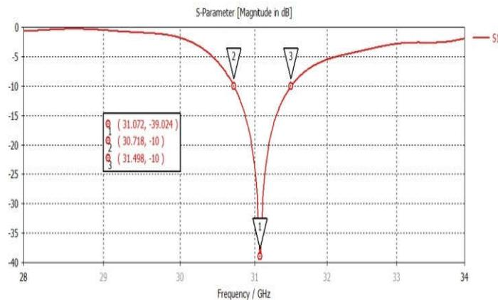
**Figure 2. Simulated S11 of the Proposed Antenna.**
