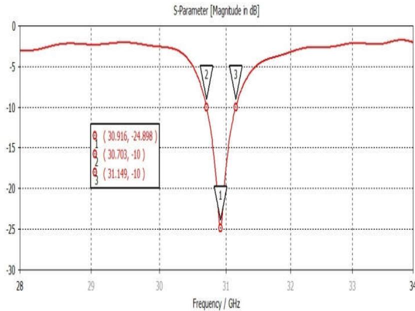
**Figure 9. Simulated S11 of the Proposed Aerial Virtual Array.**
