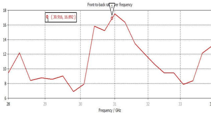
**Figure 11. Simulated Front-to-Back Ratio.**
