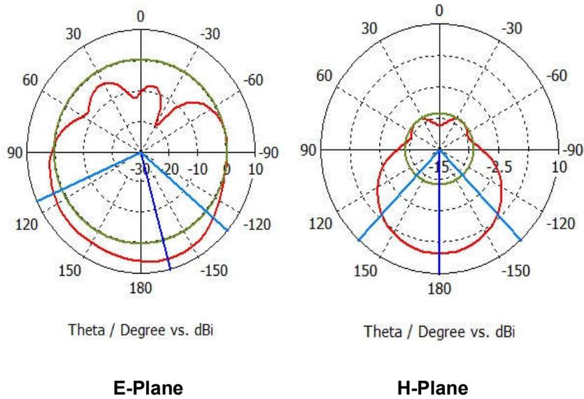
**Figure 3. Simulated Radiation Patterns in Different Cut Planes at 31.072 GHz.**
