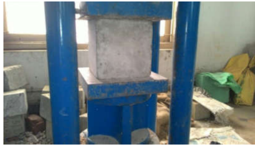
Fig. 1 Compressive Strength Test on Cubes
