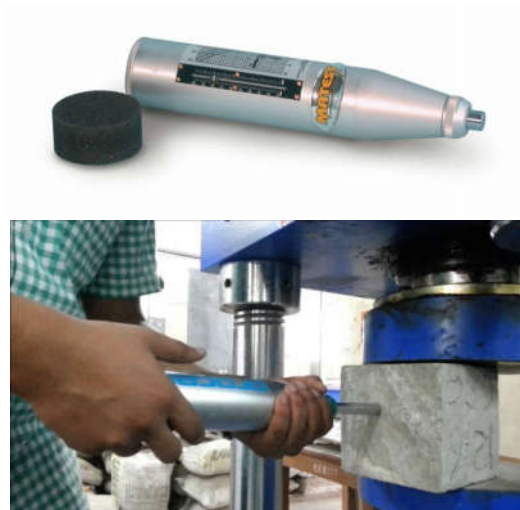
Fig.2 Rebound Hammer test
