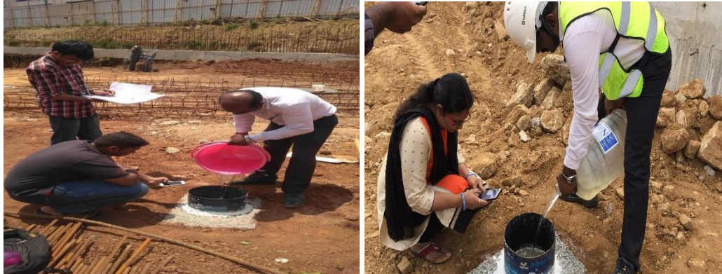
Fig 2.6 Infiltration rate Testing of Pervious Concrete Samples on Brown clay soil.
