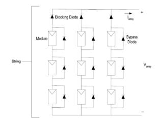
Figure 3. Layout of a PV array
