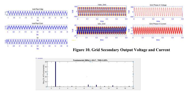
Figure 11. FFT Analysis Secondary Grid System
