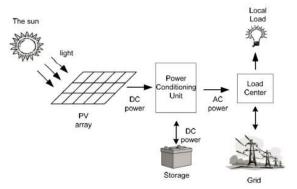
Figure 2. Main components of grid-connected photovoltaic systems
