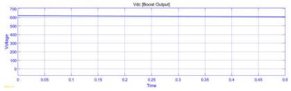
Figure 7. Boost Output Voltage
