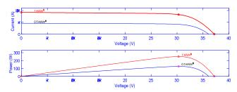
Figure 5. Matlab model I-V and P-V curves for various irradiation levels
