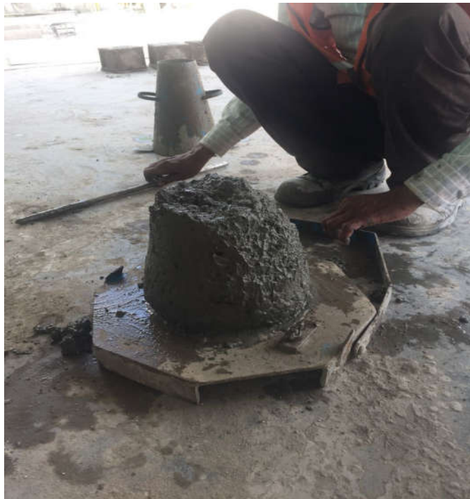
Fig. 2.6.4 (a): Slump test of concrete
