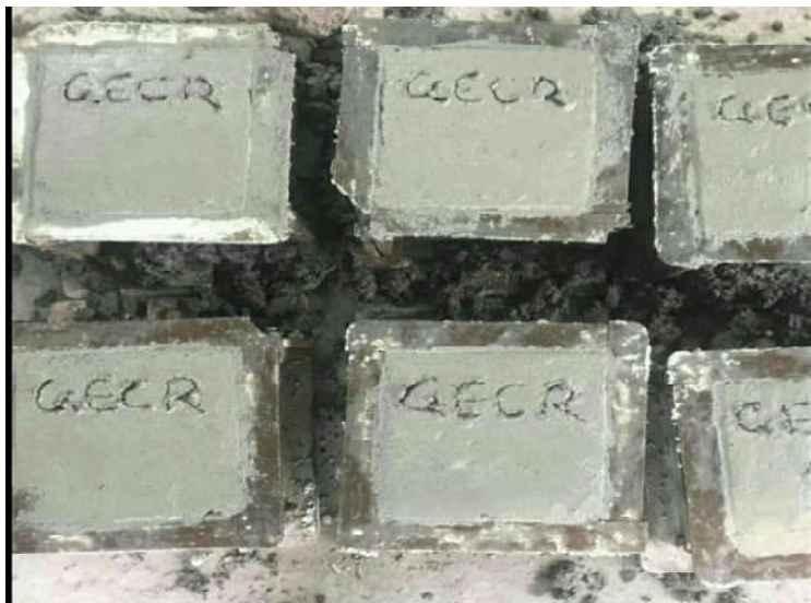
Fig. 2.6.2 (a): concrete cubes casted in the mould
