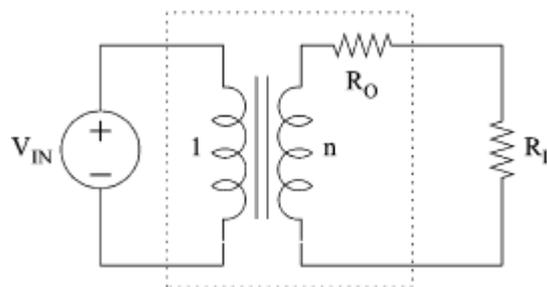
Figure 1. Model of an idealized switched capacitor converter
