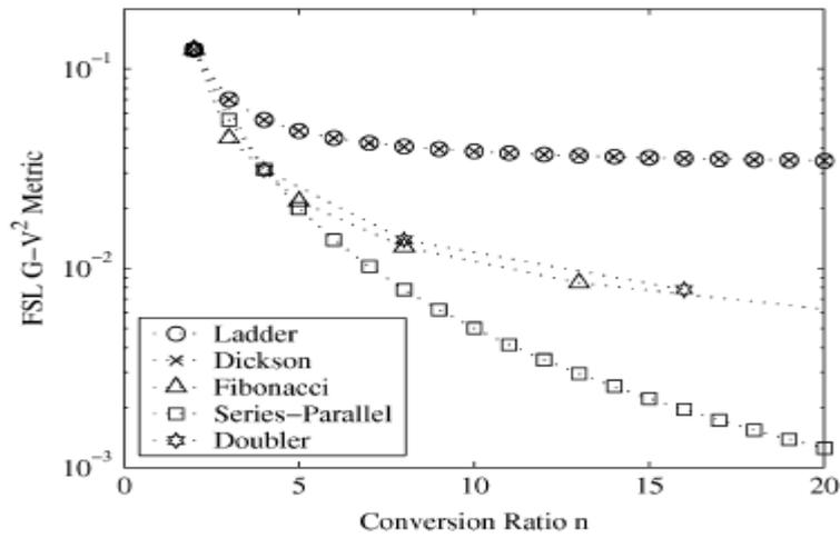
Figure 5(b). Fast Switching Limit performance scale with optimal voltage devices
