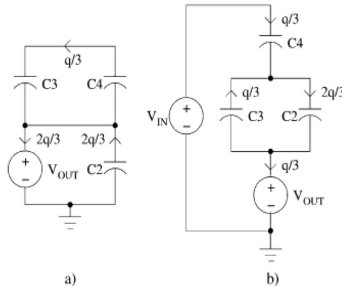
Figure 3. Charge flow in ladder converter (a) Phase 1 (b) Phase 2
