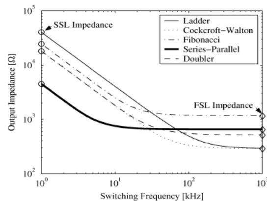
Figure 5. Simulated output impedances Vs Switching frequency
