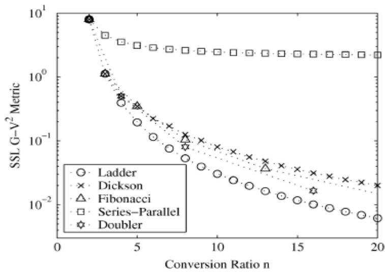
Figure 6(a). SSL performance metrics with single voltage devices
