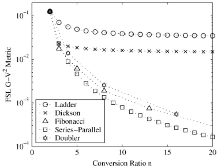
Figure 6(b). FSL performance metrics with single voltage devices
