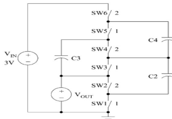
Figure 2. 3V to 1V ladder circuit
