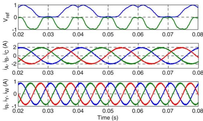
Fig. Simulation results in DF mode showing modulating references per phase, upper and lower three-phase output currents from top to bottom.
