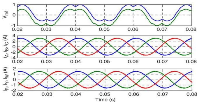
Fig. Simulation results in CF mode showing modulating references per phase, upper and lower three-phase output currents from top to bottom.
