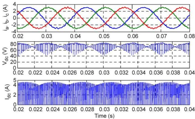
Fig. Simulation results in CF mode showing three-phase input currents ,fictitious dc-link voltage and current from top to bottom.
