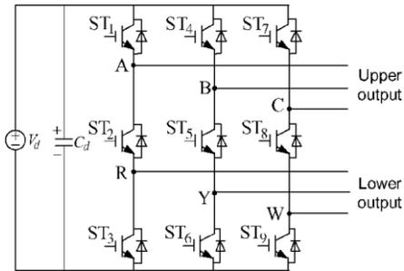
Fig. 1. Dual output nine-switch inverter.
