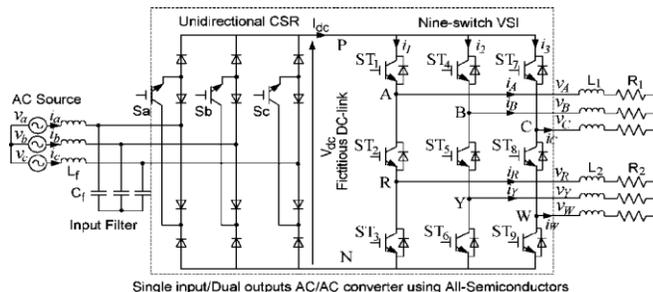
Fig 2. Topology of proposed matrix converter
