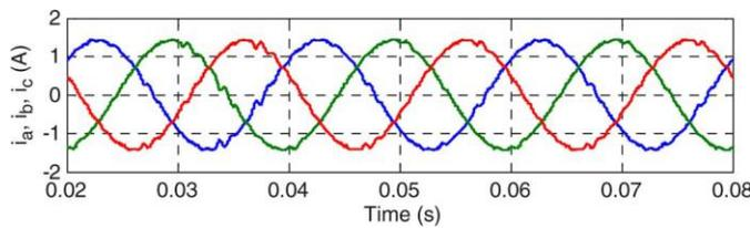
Fig. Simulation results in DF mode showing three-phase input currents.
