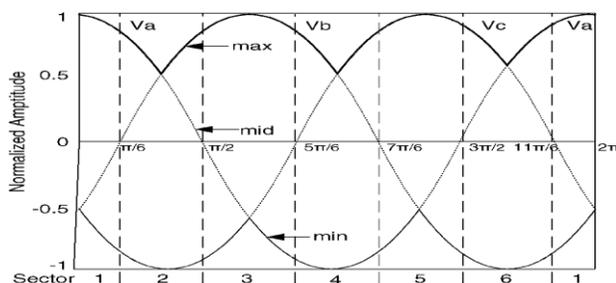
Fig 3. Six intervals of CSR input voltage waveform
