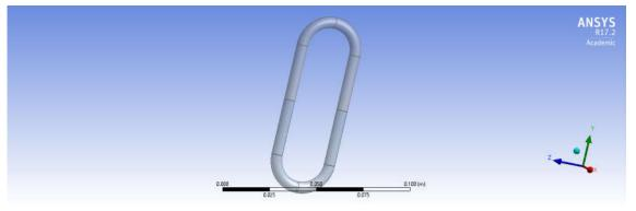
The geometry is created using CATIA V5. First, a rectangle of dimensions 30mm x 90mm is created, and then fillet is applied to each of the corners of the rectangle of radius 15mm. After this, a semicircular profile of radius 3mm is swept along this rectangle. Thus, giving the entire geometry a semicircular cross-section. It is imported to ANSYS using .igs extension.
