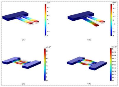
Figure 4: Finite element modeling of energy dissipation through the substrate (anchor loss) reveals a Q-factor of the anti-phase mode
