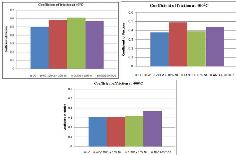
**Figure 10 Average coefficient of friction plots for uncoated and coated samples. At (a) 40°C (b) 200°C(c) 600°C**
