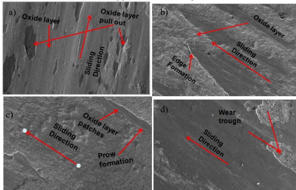
Figure 9 SEM analysis of worn out samples at 600°C (a) Uncoated specimen (b) WC-12%Co + 10% Ni (c) Cr<sub>2</sub>O<sub>3</sub> + 10% Ni (d) Al<sub>2</sub>O<sub>3</sub>-3%TiO<sub>2</sub>
