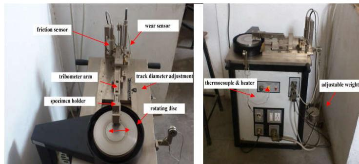
**Figure 2 Pictorial views for High temperature pin-on-disc tribometer rig.**
