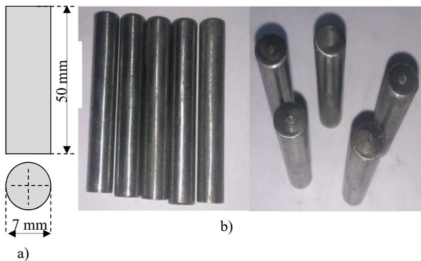
Figure 1 a) Sketch of Pin sample for wear test on pin-on-disc tribometer
