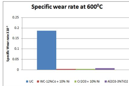
**Figure 11 Specific Wear plots for uncoated and coated samples
