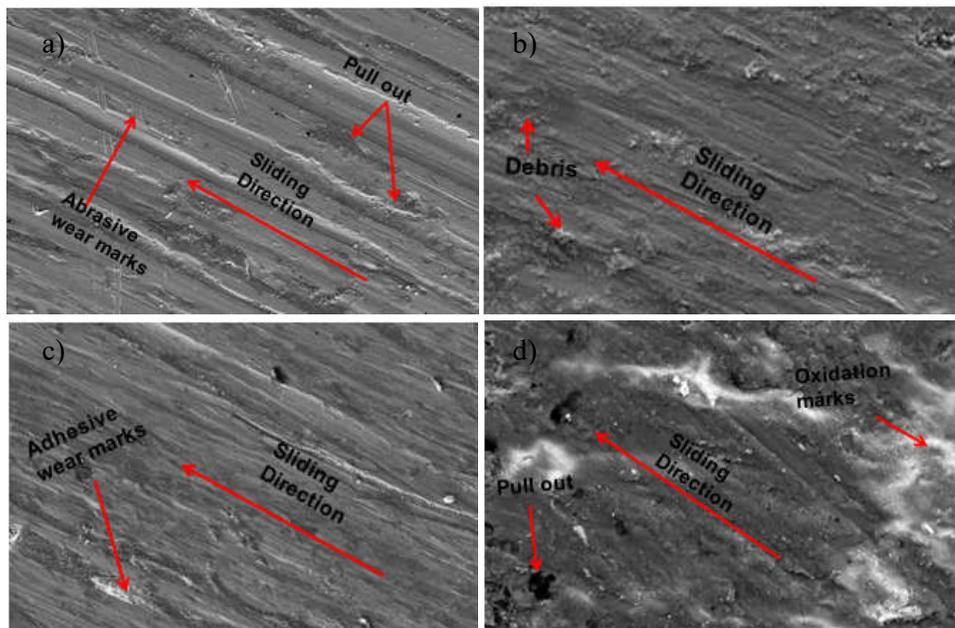
Figure 7 SEM analysis of worn out samples at 40°C (a) Uncoated specimen (b) WC-12%Co + 10% Ni (c)  $\text{Cr}_2\text{O}_3$  + 10% Ni (d)  $\text{Al}_2\text{O}_3$ -3% $\text{TiO}_2$
