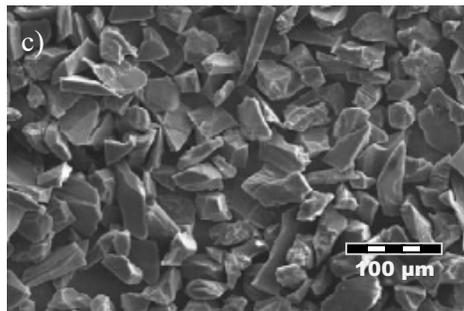
**Figure 3** SEM morphology of composite Coating powder (a) WC-12%Co + 10% Ni (b) Cr<sub>2</sub>O<sub>3</sub> + 10% Ni (c) Al<sub>2</sub>O<sub>3</sub>-3%TiO<sub>2</sub>
