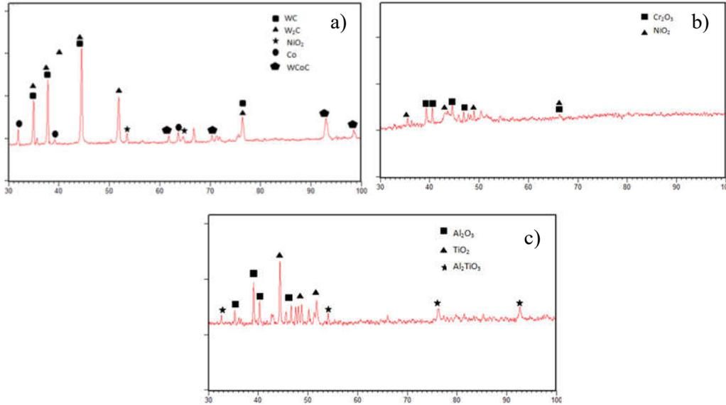
Figure 5 XRD Diffractograms (a) WC-12%Co + 10% Ni (b) Cr<sub>2</sub>O<sub>3</sub> + 10% Ni (c) Al<sub>2</sub>O<sub>3</sub>-3%TiO<sub>2</sub>
