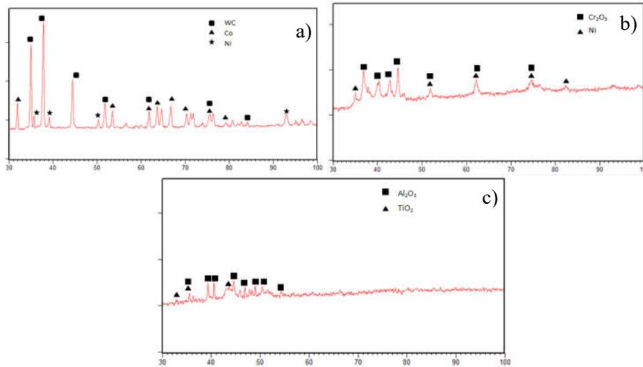
**Figure 4** XRD diffractograms of the feedstock (a) WC-12%Co + 10% Ni (b) Cr<sub>2</sub>O<sub>3</sub> + 10% Ni (c) Al<sub>2</sub>O<sub>3</sub>-3%TiO<sub>2</sub>
