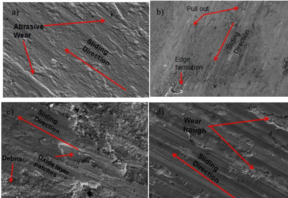
Figure 8 SEM analysis of worn out samples at 400°C (a) Uncoated specimen (b) WC-12%Co + 10% Ni (c) Cr<sub>2</sub>O<sub>3</sub> + 10% Ni (d) Al<sub>2</sub>O<sub>3</sub>-3%TiO<sub>2</sub>
