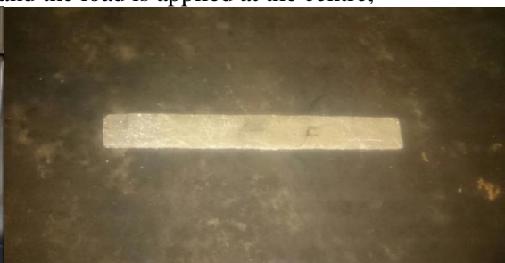
Figure 8. Flexural testing specimen
