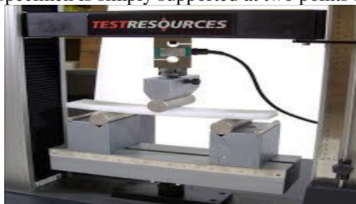
Figure 7. Flexural testing setup
