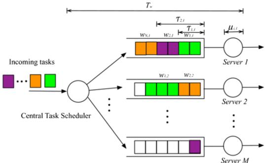
Fig 1: Mapping of various incoming jobs to different servers running as VMs on physical hosts.
