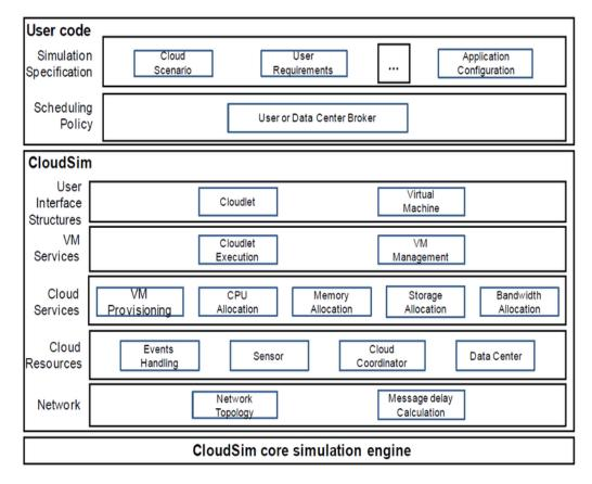
Fig 3: CloudSim architecture. User code runs on top of the Cloud simulation Engine which has the cloud infrastructure and the service details.
