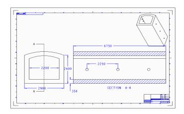
FIG 1. 7 DETAILED DRAWING HEATING CHAMBER FOR ANALYSIS
