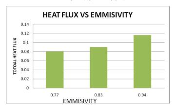
Graph 2: Graph represent radiation factor vs Heat flux distribution flow is indicated
