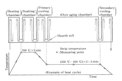
FIG 1.2 TEMPERATURE VS TIME CURVE THROUGH OUT THE PROCESS
