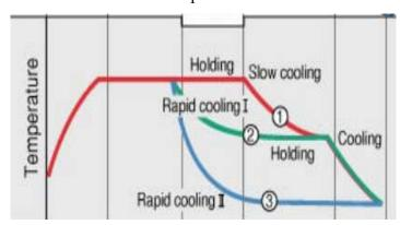
FIG 1.3 ANNEALING PROCESS(heating and cooling)
