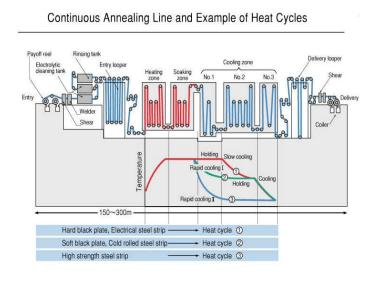
FIG 1.1 CONTINUOUS ANNEAING FURNACE WORKING PROCESS
