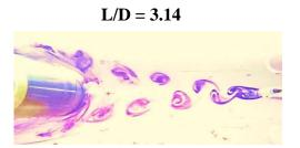
Fig.1 Flow structure at Re=1748
