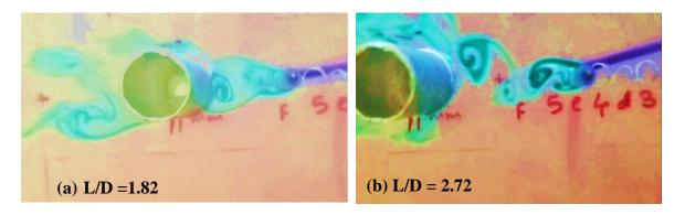
Fig.3 Flow structure at Re=745
