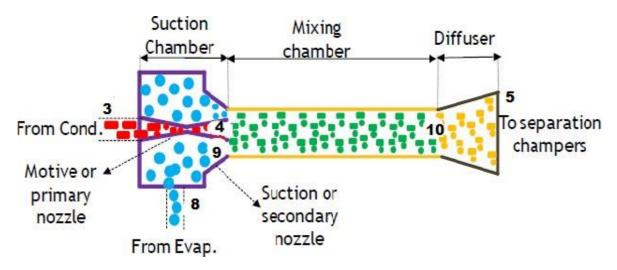
Fig 4. 7: Schematic diagram of flow inside ejector.
