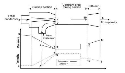
Fig 4. 2: Velocity and pressure profiles for an ejector
