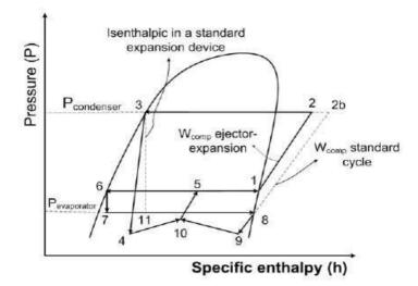
Fig 4. 3: Pressure -Enthalpy diagram of Standard cycle and EERS
