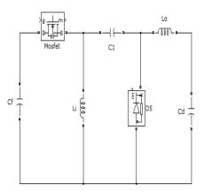
Fig. 3. Basic circuit for Zeta converter
