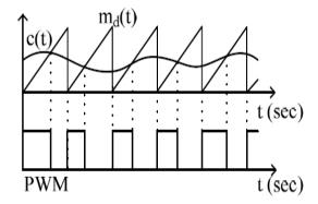
Fig. 4. Generation of PWM signal by comparing a saw tooth waveform with the controller output
