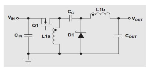
Fig. 2. Basic circuit for Zeta converter
