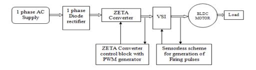
Fig. 1. Proposed Zeta converter fed Sensor-less BLDC MOTOR drive
