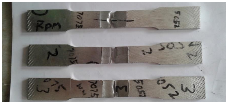
Fig 3.2 Tensile test specimen after testing
