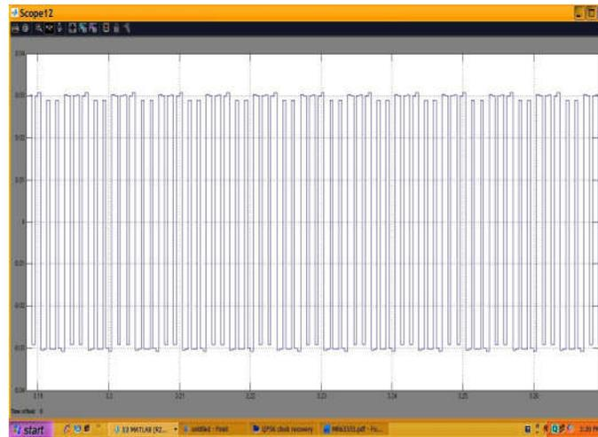
Figure 5.9. Down sampling Output for Factor of 5 in Receiver path
