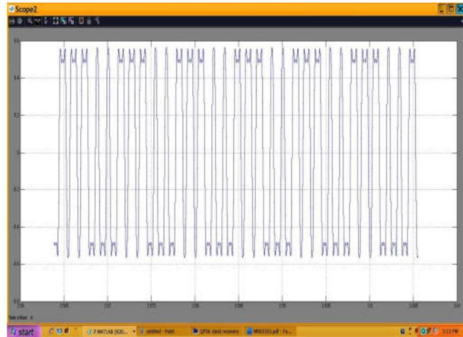
Figure 5.4. Upsampling Output for Factor of 10 in Transmission Path
