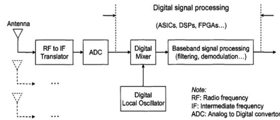
**Figure 1.1. Digital signal processing in SDR based receiver**
