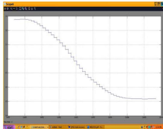
Figure 5.5. Upsampling Output for Factor of 100 in Transmission Path
