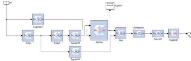
Figure 4.2. Gardner's timing error detector
