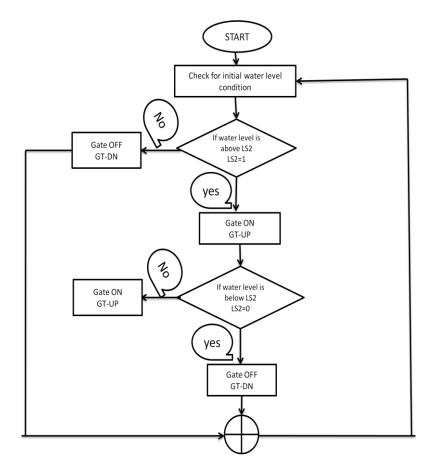
Figure 4. Flowchart of algorithm implemented
