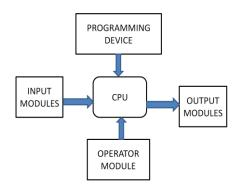
Figure 2. Block diagram of PLC
