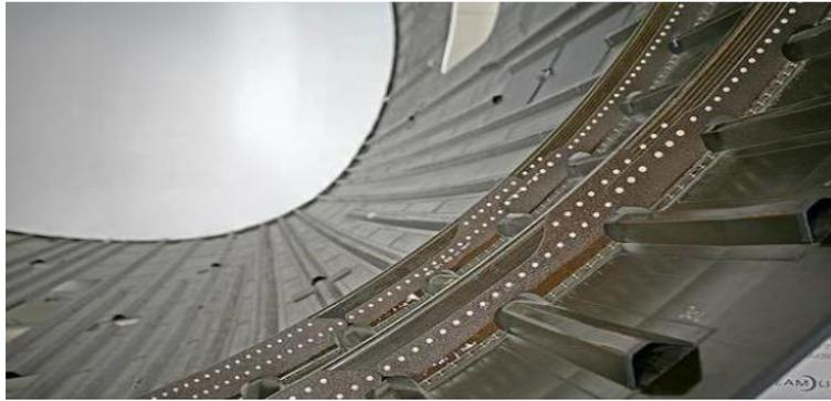
Fig. 4: Composite fuselage with hat cross section [7]
