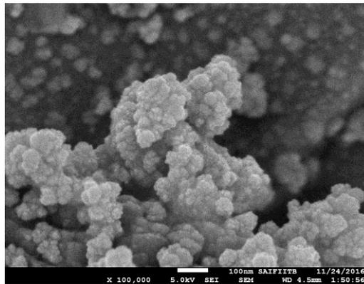
Figure 1 SEM image for La and Sn doped cadmium Sulphide nanoparticles
