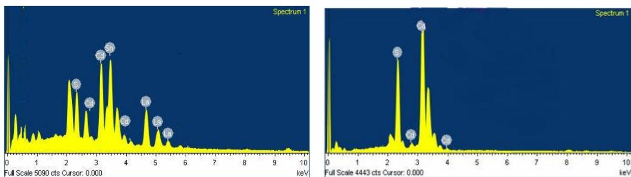
Figure 3 EDX image of a. La and Sn doped CdS b. Pure CdS
