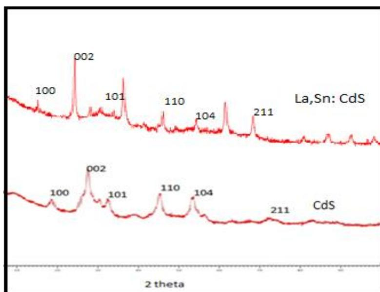
Figure 4 XRD pattern of La and Sn doped CdS and pure CdS nanoparticles
