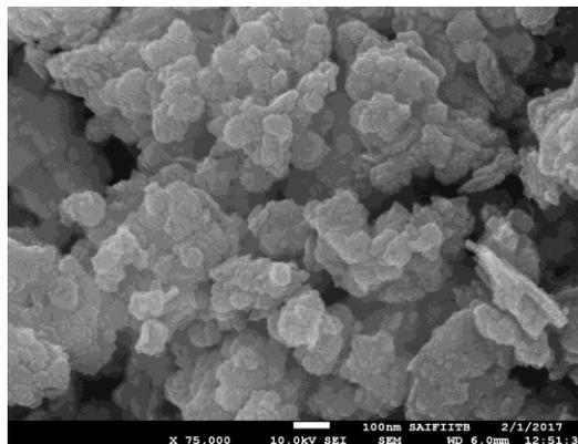
Figure 2 SEM image for pure Cadmium sulphide nanoparticles
