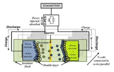
Fig.2 The capacitor storage system [10].
