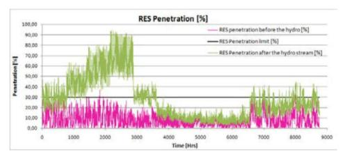
Fig. 9 The RES penetration with the SHPP.
