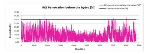
Fig.8The RES penetration from Wind and SPVs.
