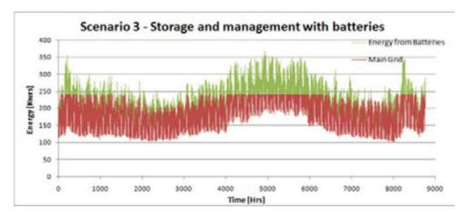
Fig.7 The Energy Demand with Batteries.
