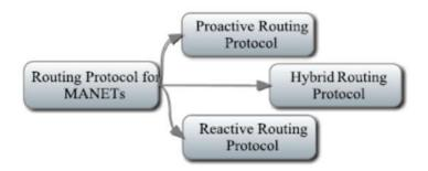
Fig. 2 Routing Protocols for MANETs
