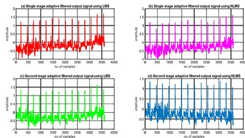
**Fig. 4:** Simulation results of MA Cancellation for MIT-BIH Record Number 105 (a) Recovered (red) signal using SSLMS algorithm (b) Recovered (green) signal using TSLMS algorithm (c) Recovered(magenta) signal using SSNLMS algorithm (d) Recovered(blue) signal using TSNLMS algorithm
