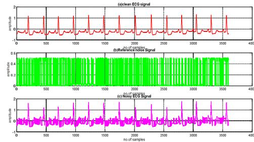
**Fig. 3:** Simulated model filtering results of MA Noise Cancellation (a) Clean ECG Signal(red) for MIT-BIH Record Number 105 (b) Reference Ma Noise Signal (green) (c) MIT-BIH Record 105 with MA noise (magenta)
