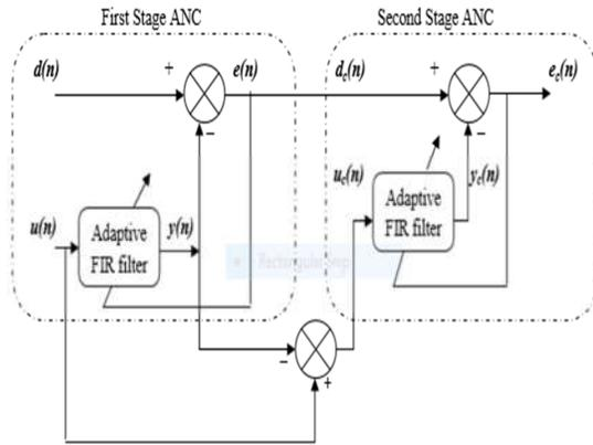
Fig. 2: Proposed Two Stage Adaptive Noise Canceller for ECG denoising
