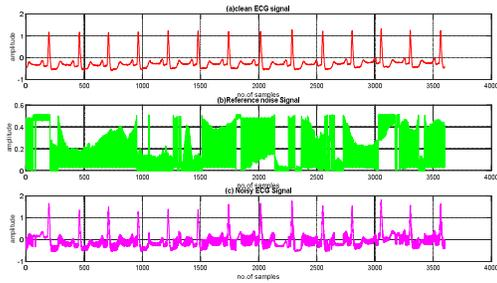
**Fig. 5:** Simulated model 1 filtering results of EM Cancellation (a) Clean ECG Signal (red) for MIT-BIH Record Number 105 (b) Reference EM noise signal (green) (c) MIT-BIH Record 105 with EM noise (magenta)
