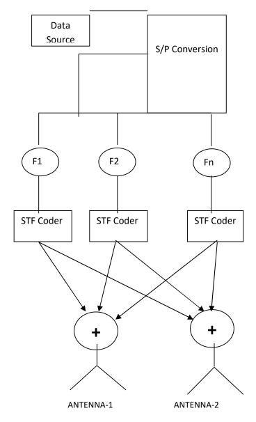
Fig.1. System Model for Separate STF coding rule
